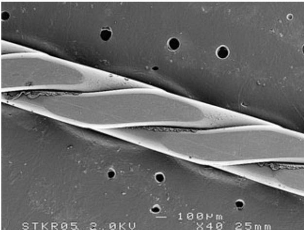
**Fig 2e** Quad Cat stainless-steel wire (original magnification 40X).
