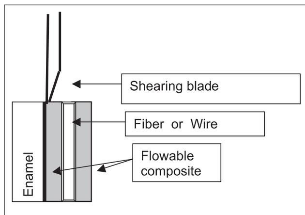
**Fig 4a** Schematic drawing of the cross-section of a specimen showing FRC or wire in relation to their application modes and the position of the shearing blade of the universal testing machine.
