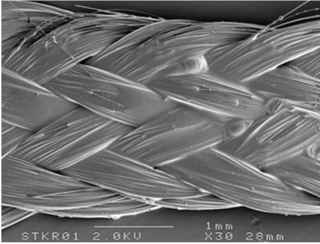
**Fig 2a** Representative SEM image of Angelus Fibrex Ribbon (original magnification 80X).
