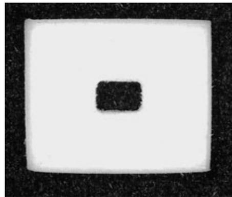
**Fig 3** Rectangular polyethylene mold (3.2 x 2.2 x 1.5 mm) used for positioning the retainer and the flowable resin in a controlled manner.
