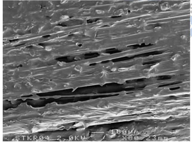
**Fig 2b** Representative SEM image of DentaPreg Splint (original magnification 80X).
