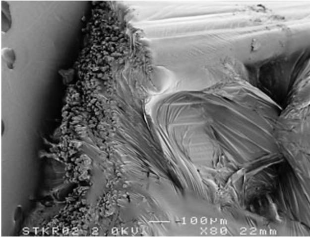
**Fig 2c** everStick Ortho (original magnification 80X). Note the resin impregnation of the fibers on as-received samples.
