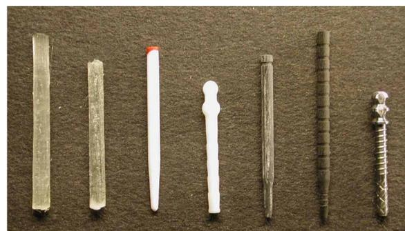
Figure 1. Posts used in the study. From the left: Stick, everStick, Snowpost, ParaPost FiberWhite, C-Post, C-Post serrated and ParaPost XT.
