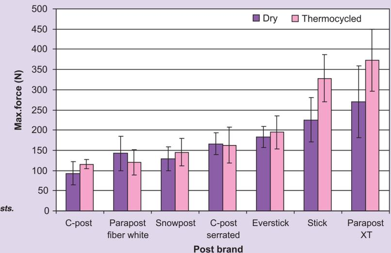
Figure 6. Mean Pull-out forces and standard deviations for studied posts.
