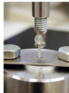
Figure 4. The custom-made jig for measuring the Pull-out force for posts.
