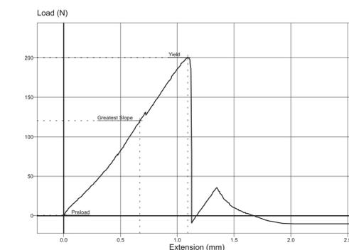
Figure 5. The loading curve for measuring the Pull-out force of everStick post.
