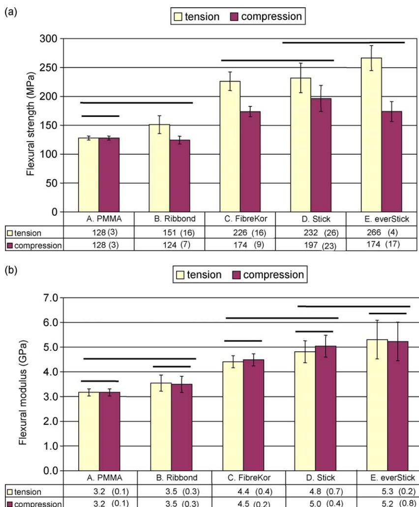
**Figure 2** (a) Three-point flexural strength and (b) calculated three-point flexural modulus of the test specimens reinforced with various brands of fiber reinforcements and two fiber locations (compression or tension side). Vertical bars represent SD. Horizontal lines above the bars indicate groups that do not differ statistically from each other.
