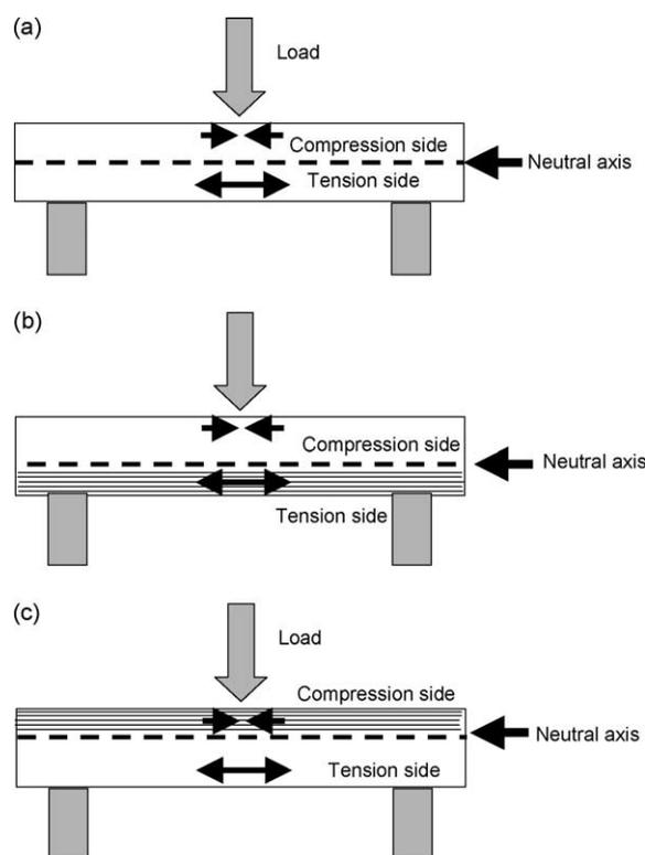
**Figure 3** Schematic representation of highlighting the areas of tensile and compression side. If specimen is homogenous without any reinforcement, neutral axis located in the middle of test specimen (a), but if the fiber reinforcement is placed in tension side of the test specimen (b), or in the compression side (c), neutral axis is moved towards fiber reinforcement layer.
