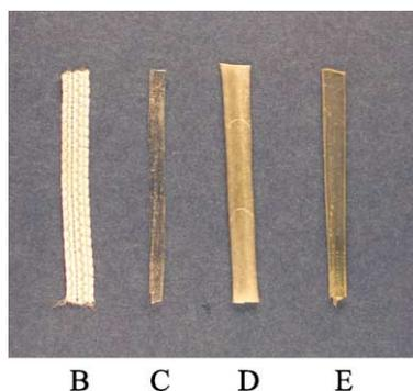
**Figure 1** Fiber reinforcements used in test groups in the current study. Group (B) Ribbond; Group (C) FibreKor; Group (D) Stick; and Group (E) everStick fiber reinforcement.
